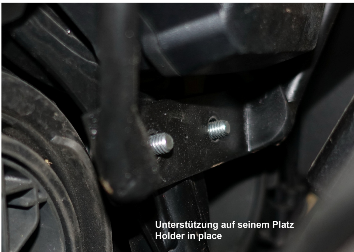
Die Unterstüztung ven unten nach oben gleiten. Put the holder in a lower position until the upper parts are close to the frame and then slide it upwards to it's position.
